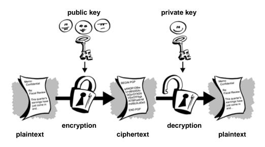
Figure 3-1. Public Key Cryptography diagram
